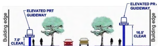
Figure 9. Potential elevated guideway
