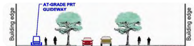
Figure 8. Potential at-grade guideway
