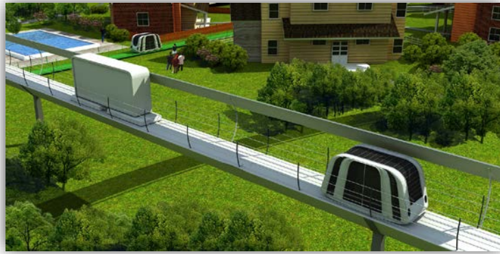
Passenger and goods vehicles use the same infrastructure. Note the solar panels shading the vehicles
