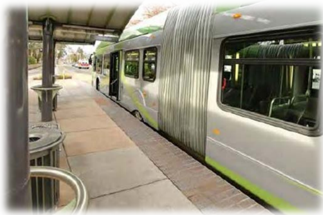
BRT Level boarding platform Source: GCEDC 2010 Multimodal Transit Corridor Alternatives Feasibility Study
