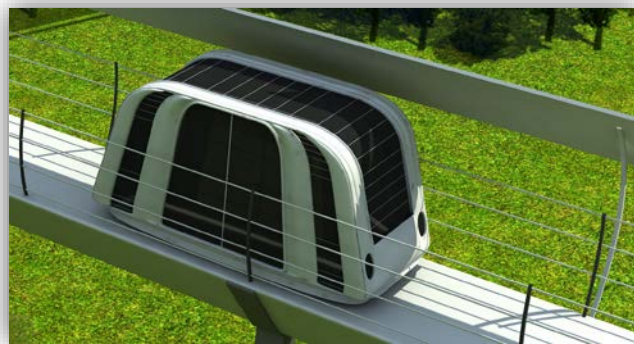
Solar panels also help shade the vehicles
