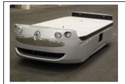
Figure 21 - FRT for delivery of small goods and removal of waste (not yet in service).
