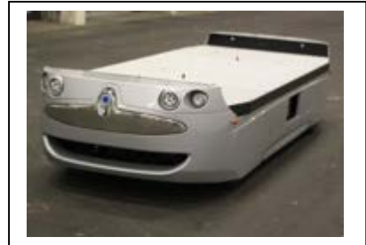
Figure B-9: FRT for delivery of small goods and removal of waste (not yet in service).
