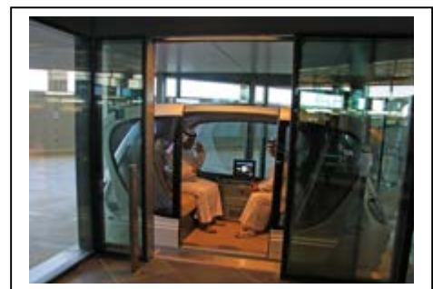
Figure B-11: Masdar station level platform with 4 passenger vehicles, seated across.
