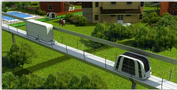
Passenger and goods vehicles use the same infrastructure. Note the solar panels shading the vehicles
