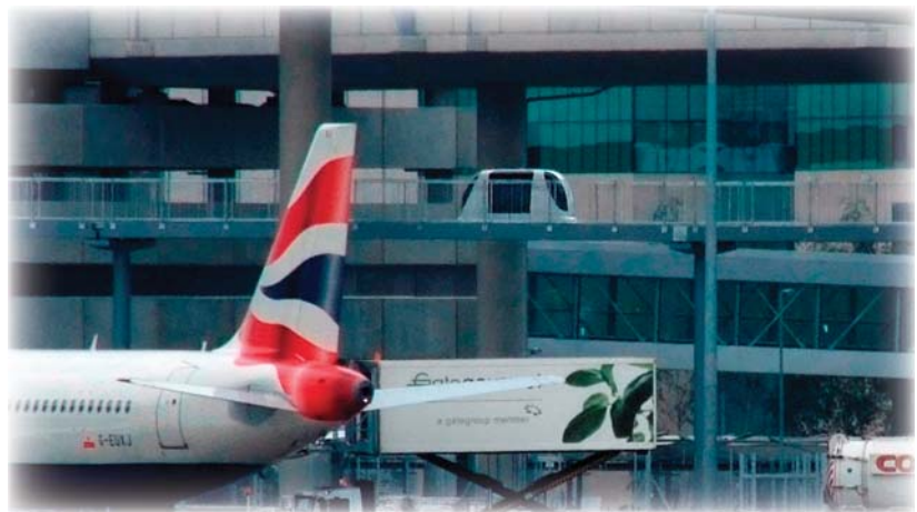
T-Pod and guideway under T5 access road
